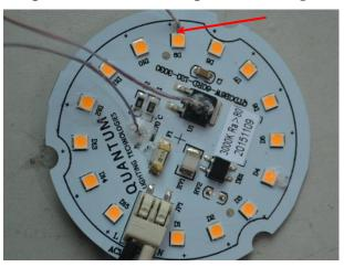
Temperature measurement point of LED light source  $(TMP_b)$
