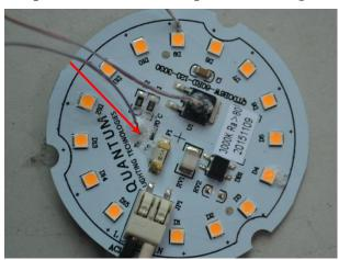
Temperature measurement point of driver (TMP<sub>c</sub>)
